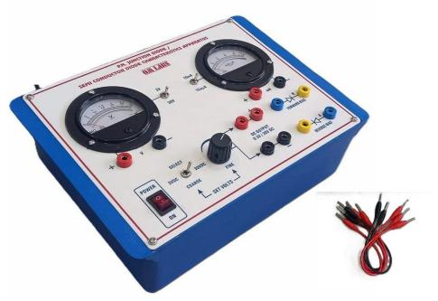
P N Junction/ Semi Conductor Diode Characteristics Apparatus is used for doing the practical of PN Junction Diode in Forward & Reverse Bias
